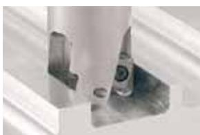
After end milling for a distance of 200 feet, a fine surface finish of Ry 4.3μm was achieved and maintained, including the corner radius.
