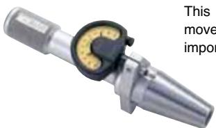
This is the arbor used to measure the axial movement of the holder on clamping, which is important for BIG-PLUS®.
